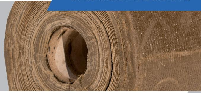
**Denso Tape** is composed of a non-woven synthetic fabric carrier, fully impregnated with a neutral compound based on saturated petrolatum and inert siliceous fillers. **Denso Tapes** are designed to withstand extreme temperature variations. The tapes provide long term corrosion protection to pipes, flanges, valves and related surfaces. The tapes too seal and water proof metal both above and below ground.
