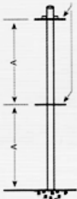
Fig 3: Tall Column Bracing Bracing for tall columns where already erected building framing or scaffold is available for support.
