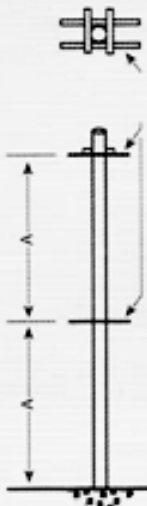
Fig 1: Columns on a line Bracing for relatively short columns – where height to diameter does not exceed 12 to 1.
